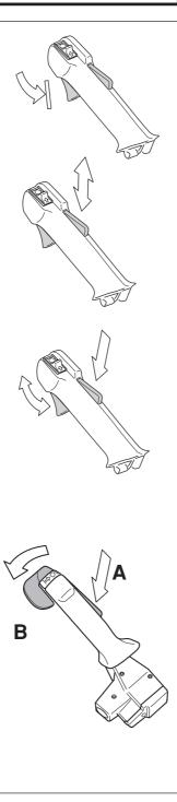
• See section "*Start*". Start the machine and apply full throttle. Release the throttle and check that the cutting equipment stops and remains at a standstill. If the cutting equipment rotates with the throttle in the idling position then the carburettor's idling setting must be checked. See chapter *"Maintenance"*.
